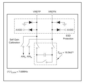
Figure 12. Simplified Reference Input Circuitry
