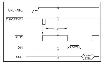
Figure 18. Data Retrieval After Synchronization
