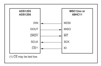
Figure 28. Connection to Microcontrollers with an SPI Interface
