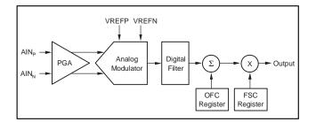
Figure 23. Calibration Block Diagram
