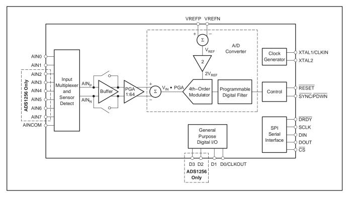
Figure 5. Block Diagram
