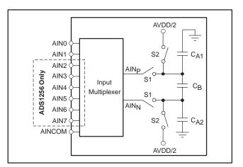
Figure 9. Simplified Input Structure with Buffer Off
