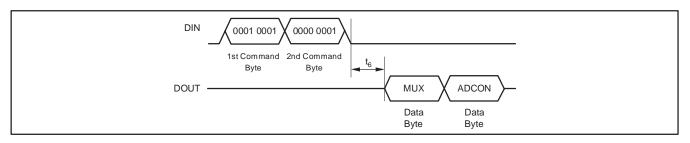
Figure 34. RREG Command Example: Read Two Registers Starting from Register 01h (multiplexer)
