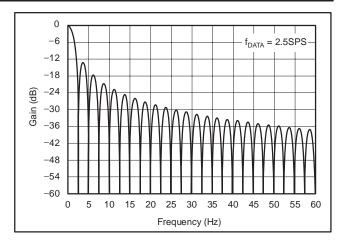
Figure 15. Frequency Response for Data Rate = 2.5SPS
