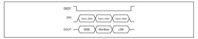
Figure 32. DIN and DOUT Command Sequence During Read Continuous Mode
