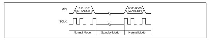
Figure 37. STANDBY Command Sequence
