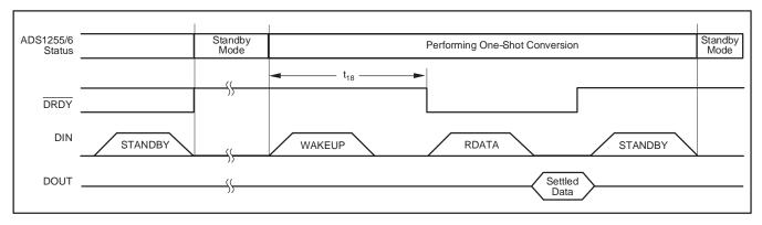
Figure 20. One-Shot Conversions Using the STANDBY Command
