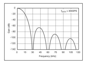
Figure 14. Frequency Response for Data Rate = 30kSPS
