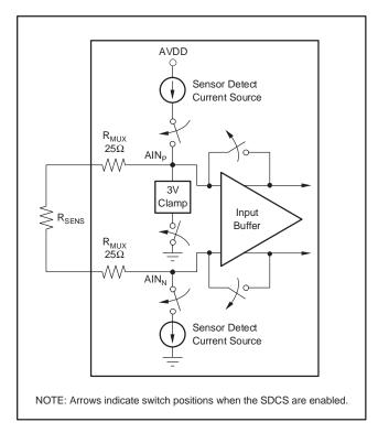
Figure 7. Sensor Detect Circuitry
