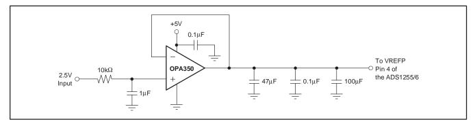
Figure 26. Recommended Voltage Reference Buffer Circuit
