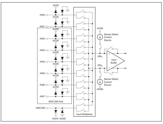
Figure 6. Simplified Diagram of the Input Multiplexer
